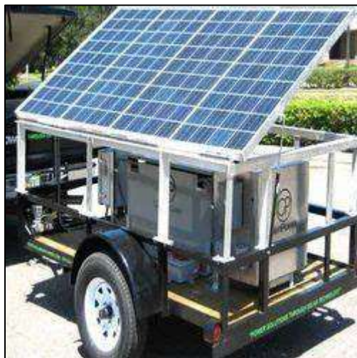
Fig 1: Solar powered Generator for Tractors Source: https://dir.indiamart.com
